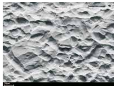
Standard quality tube annealed, chemically descaled, pickled roughness ID Ra approx. 2.5 µm
