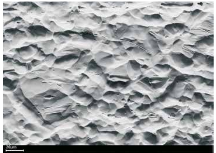
pickled inside surface Roughness Ra. approx. 2.5 µm 500-fold magnification
