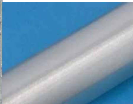
surface ground by 320 grit roughness Ra approx. 2,0 µm
