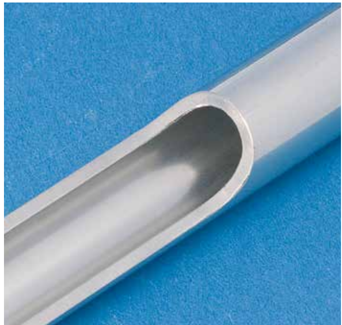
TPS standard SBS Level 2: bright annealed surface outside inside roll polished and bright annealed roughness outside Ra max. 0,8 µm | roughness inside Ra max. 0,8 µm
