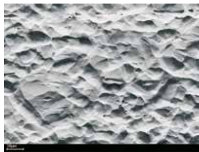
Standard quality tube annealed, chemically descaled, pickled roughness ID Ra approx. 2.5 µm
